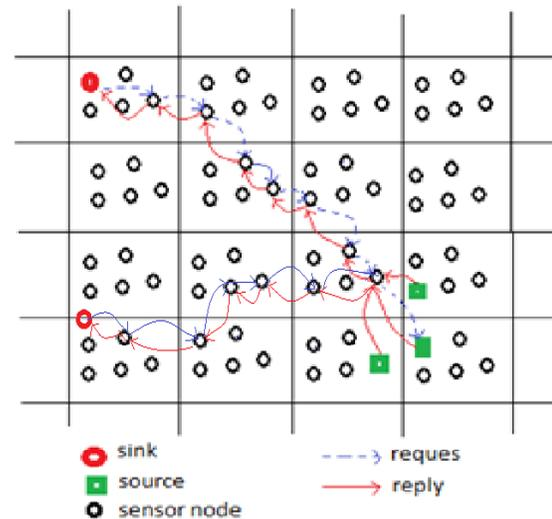
**Figure 2:** Sink request and source reply process
